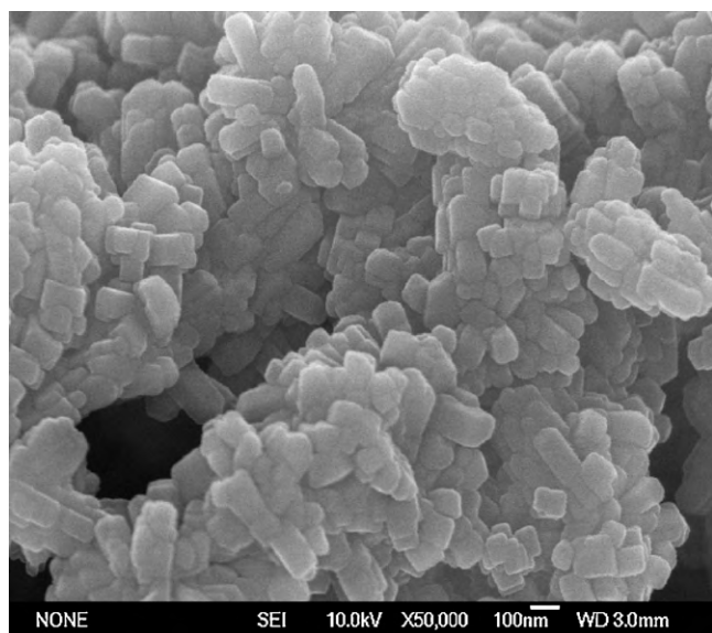
Fig. 2. High-resolution SEM (S-2700) image of nano-scale HZSM-5.
